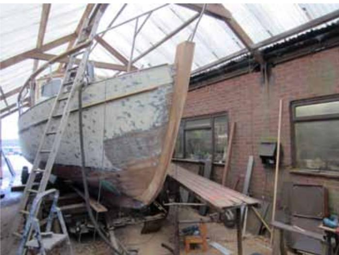
After a long winters work replacing the stem, scarping in 5 plank ends on each side, numerous parts of frames, 4 beam shelf ends, together with the multitude of other maintenance
